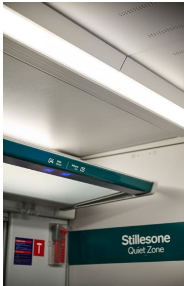
The new led lights have a brighter and whiter light, and last longer than the old ones.
